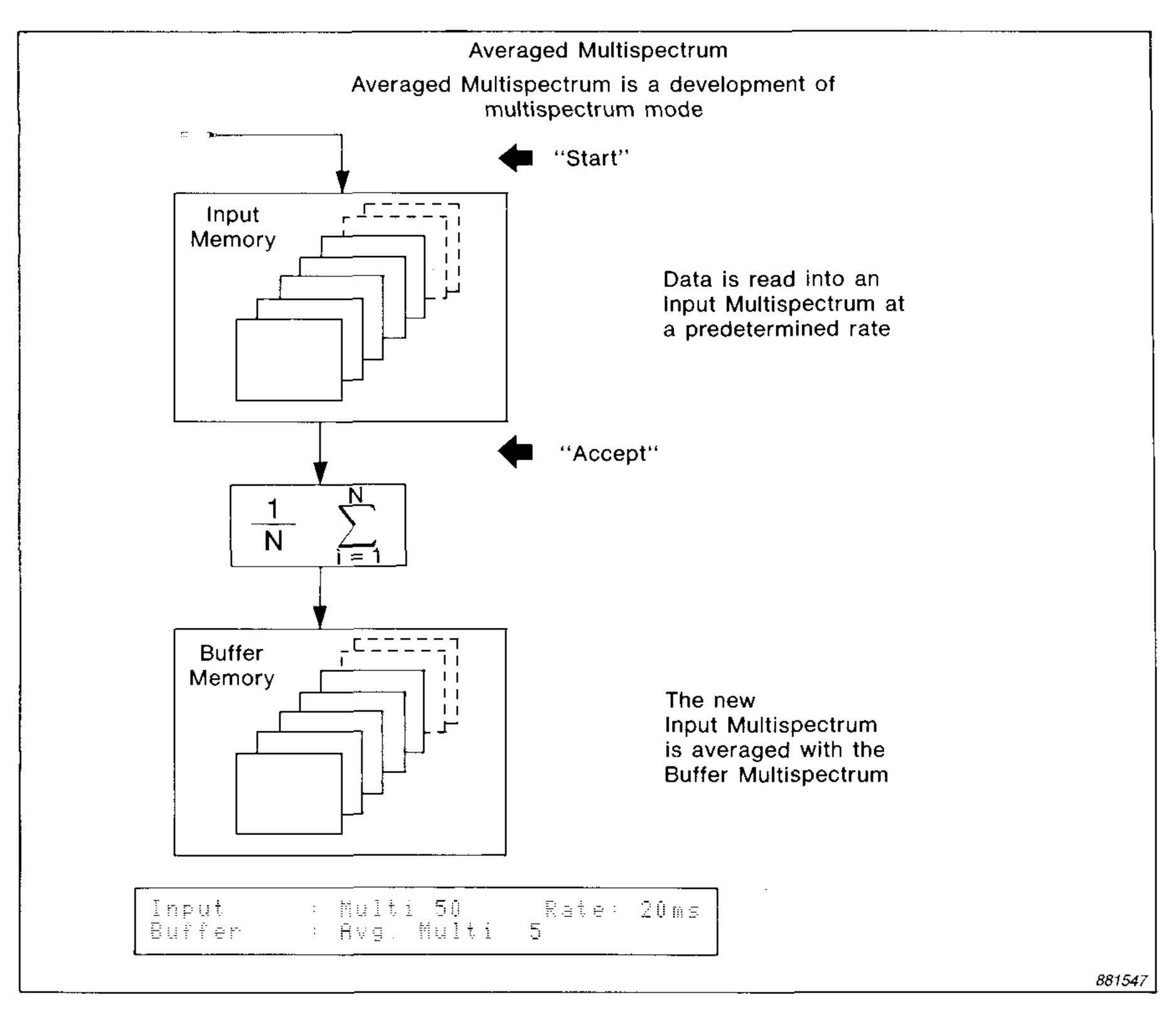
multispectrum, which is the average of the five measurements, is stored in the buffer memory.
