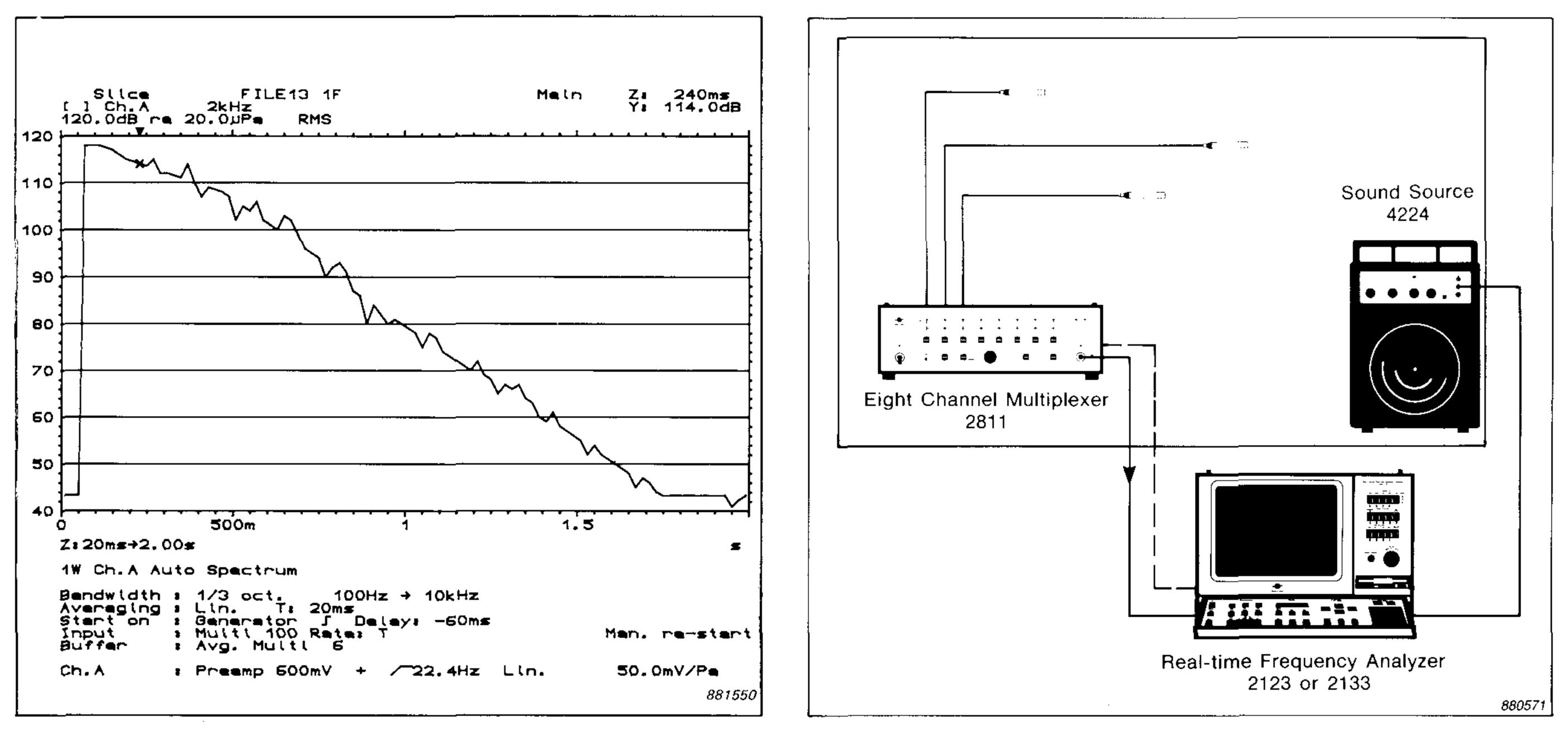
Fig. 3. Typical measurement set-up for a reverberation time measurement using interrupted noise
